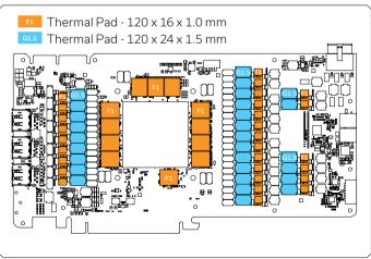
Your EK-Quantum Vector<sup>2</sup> Strix/TUF RTX 3090 Ti D-RGB block comes with Thermal Pads that have to be cut into smaller pieces to cover all the VRM components. EK made sure to provide you with more than an adequate quantity of Thermal Pads to complete this Step.
