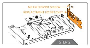
Position the replacement I/O Bracket on the water block. During this process, make sure you have aligned the holes. Secure it with the two (2) M3 x 6 DIN7991 Screws and Allen Key 2 mm.
