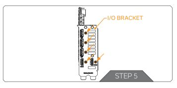
Lastly, unscrew four (4) Screws and detach the I/O Bracket (using Phillips head screwdriver).
