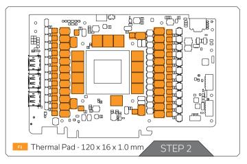
Once cut to the size, Thermal Pads should be placed on the PCB, as shown in the picture:
