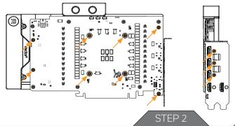
Use seven (7) M2.5 x 4 AX1 Screws and PVC washers to tighten the PCB on the water block. Tighten the screws evenly using the Phillipshead screwdriver. An additional one (1) M2.5 x 6 AX1 Screw must be secured with an M2.5 Nut.
