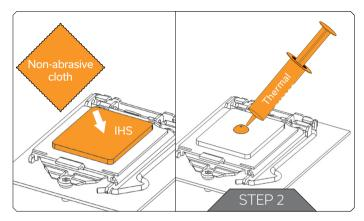
**Cleaning the CPU:** Wipe the CPU's contact surface (by using non-abrasive cloth or Q-tip, as shown on sample photo).
