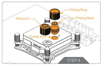
Tighten the fitting barbs in clockwise direction until the gasket underneath is compressed.
