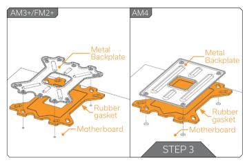
Install backplate rubber gasket and place metal backplate for AMD® socket to the back of your motherboard RIBBED SIDE UP! (facing away from the motherboard) Align the holes on the motherboard with holes on rubber gasket and backplate.
