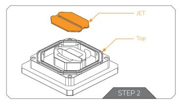
Unscrew the four M4 screws in counter-clock-wise direction from the bottom of the water block using enclosed 2,5mm Allen key to release the assembly, consisting of water block top and jet plate. Upon replacing the jet plate please reassemble the water block as shown on the in STEP 1 and STEP 2 pictures. Pay special attention to the insert orientation relative to the copper base and water block top!
