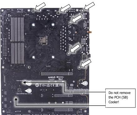
Removing of the original plastic hold-down clamps and the factory backplate: Using Philips-head screwdriver remove the four UNC 6-32 screws securing the original plastic hold-down clamps around the socket as shown on the sketch. Remove the original AMD® backplate and the hold-down clamps and store them away.
