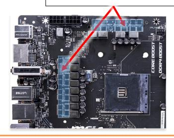
Replacement thermal pads @ EKWB web shop: Thermal PAD F 0.5mm - (120x12mm) [EAN: 3830046996725]
