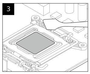
Ensure every part of the die area is covered with a thin layer of thermal compound.
