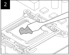
Use the included plastic brush to spread the compound equally over the surface for maximum coverage.
