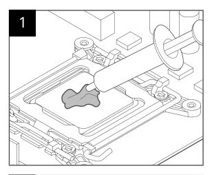
Clean off any dust or existing thermal compound on the surface, then squeeze a small drop (pea size) of your new compound on the center of the CPU.
