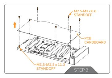
Unscrew seven (7) M2.5-M3 x 6.6 standoffs with the included tool (EK-Plug out Spludger Tool). Make sure not to unscrew the M3.5-M2.5 x 11.3 standoffs! In case the M3.5-M2.5 x 11.3 standoff unscrews, carefully tighten it back with the 4 mm wrench.
