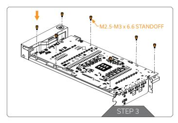
Place the M2.5-M3  $\times$  6.6 Standoff in each of the seven (7) mounting holes of the standoff M3.5-M2.5  $\times$  11.3 (as shown in the image) and tighten them evenly with the EK-Plug-Out Spludger Tool.
