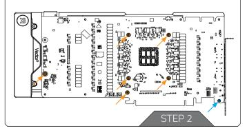
After placing the water block, use six (6) M2.5 x 4 AX1 screws and PVC washers to tighten the GPU PCB. Tighten the screws evenly using the Phillips-head screwdriver. EK recommends you start tightening the screws around the GPU core first and then continuing outward to prevent damaging the GPU. Always use a plastic washer under each screw.
