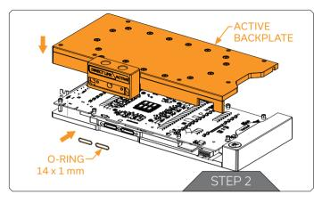
Put two O-rings  $14 \times 1$  into slots on the cold plate. Then carefully place the active backplate on standoffs as shown in the image. While putting the active backplate on the PCB, make sure the O-rings stay in the slots.
