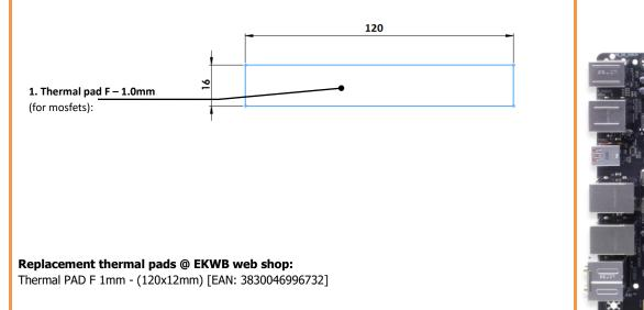
Place 1mm thermal pads (1) in larger strips over marked area and make sure all mosfet chips are covered.
