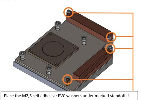
**STEP 4: ATTACHING BLOCK ON TO THE MOTHERBOARD**
