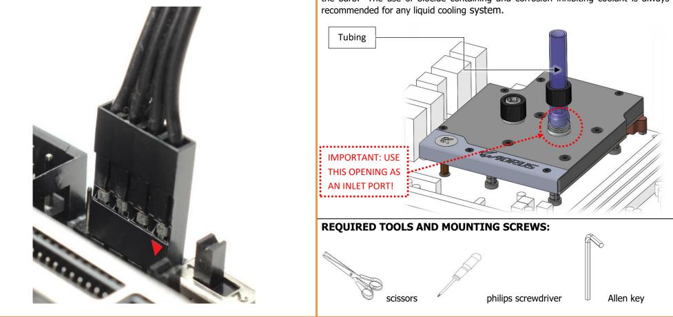
For the EK-FB GA AX370 Gaming Monoblock series water block to operate properly the G1/4 port nearest to the right edge of the water block MUST BE USED AS THE INLET PORT. EK recommends the use of EK-ACF fittings. When using fittings other than EK-ACF series please use hose clamps or appropriate substitute to secure the tubing to the barb. The use of biocide containing and corrosion inhibiting coolant is always
