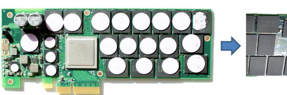
2. APPLYING THERMAL COMPOUND. Wipe off the remains (by using non–abrasive cloth or *q-tip*) of the original thermal compound until the components and circuit board are completely clean. Apply thermal compound: lightly coat chip with enclosed EK-TIM Ectotherm thermal grease. EKWB recommends to apply thermal grease in cross form for best performance (see sample picture).
