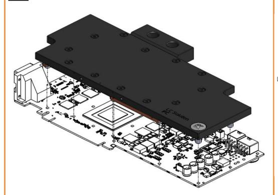
3. ATTACHING BLOCK TO GRAPHIC CARD. By using Philips screwdriver screw in enclosed M3x4 DIN7985 screws. EKWB recommends users to start tightening the screws around the GPU core and continue outwards. <u>Always use</u> a plastic washer
