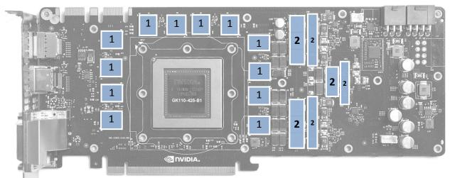
2. PLACING BLOCK TO GRAPHIC CARD. Carefully position the water block with preinstalled 2.5 mm standoffs on to the graphics card. During this process please make sure you align mounting holes on PCB with holes on the water block. Also pay attention not to use too much force by pressing block down to PCB. Chip dies are prone to cracking. We recommend completing STEP 5 prior to attaching the water block!
