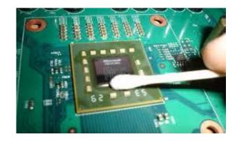
3. APPLYING THERMAL COMPOUND. Wipe off the remains (by using non–abrasive cloth or *qtip*) of the original thermal compound until the components and circuit board are completely clean. Apply thermal compound: lightly coat *NVIDIA* GPU chip with enclosed EK-TIM Ectotherm thermal grease. EKWB recommends to apply thermal grease in cross form for best performance (see sample picture).
