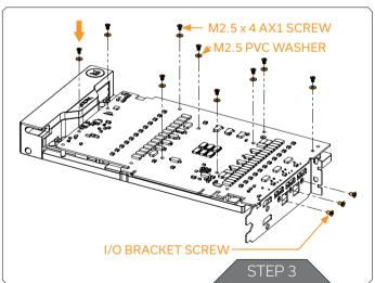
Carefully place the water block with preinstalled standoffs and replacement I/O Cover on the GPU PCB. During this process, make sure you have aligned the mounting holes of the PCB with the holes of the water block.
