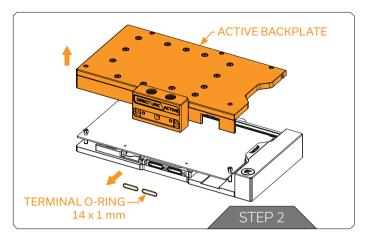
Carefully remove the complete active backplate with the terminal. Additional two (2) O-rings 14 x 1 mm needs to be removed.
