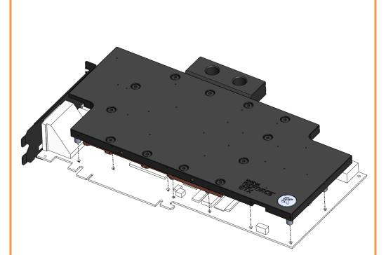
2. ATTACHING THE BLOCK TO THE GRAPHIC CARD. Use a Philips screwdriver screw with the enclosed M2,5x4 AX1 screws. EKWB recommends users to start tightening the screws around the GPU core and continue outwards. <u>Always use</u> a plastic washer under each and every screw! If the washer is already present on the circuit board (usually around the four GPU core screw holes) there is no need for additional washer. Enclosed M2x5 and M2 nut is for securing the I/O bracket as shown on picture below.
