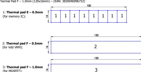
4. PLACING THERMAL PADS ON PCB. Place thermal pads on the circuit board as shown on the picture below. Refer to numbering in previous picture when applying thermal pads of different sizes or thicknesses. EK made sure to provide customers with more than adequate quantity of thermal pads to complete this step.
