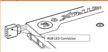
Plug the 4-pin connector from Water block's RGB LED light to the RGB\_HEADER on the motherboard. The LED will work if the pin layout on the header is as follows: <u>+12V G R B</u>.
