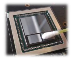
2. APPLYING THERMAL COMPOUND: Apply thermal compound: lightly coat *HBM* chip with enclosed EK-TIM Ectotherm thermal grease. EKWB recommends to apply thermal grease in cross form on the GPU area and line form on the memory area for best performance (see sample picture).
