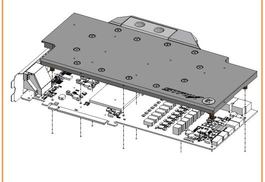
2. ATTACHING THE BLOCK TO THE GRAPHIC CARD. Use a Philips screwdriver screw with the enclosed M2,5x4 AX1 screws. EKWB recommends users to start tightening the screws around the GPU core and continue outwards. Always use a plastic washer under each and every screw! If the washer is already present on the circuit board (usually around the four GPU core screw holes) there is no need for additional washer.
