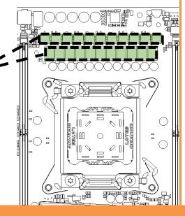
PLACING THE BLOCK ON THE MOTHERBOARD. Place the EK-FB MSI X299 GAMING PRO CARBON RGB Monoblock series water block gently to the motherboard or vice versa (as shown on photo below). Make sure that mounting holes are aligned.
