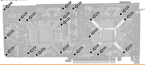
2. CLEANING THE PCB. Carefully detach the original stock cooler after removing **all** screws securing it to the board. Wipe off the remains (by using non–abrasive cloth or *qtip*, as shown on sample photo) of the original thermal compound until the components and circuit board are completely clean. EKWB recommends the use of denatured alcohol for removing TIM leftovers.
