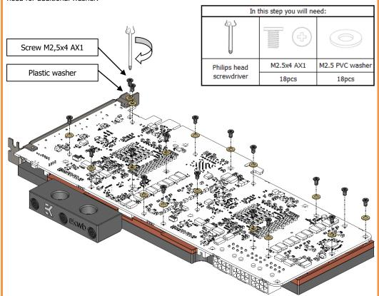
4. (OPTIONAL) ATTACHING THE FACTORY BACKPLATE TO THE GRAPHIC CARD: Please remove 3 (three) M2.5x4 AX1 screws and PVC washers that correspond to the holes of factory provided backplate. Use a Philips screwdriver with the enclosed 3 (three) M2.5x6 AX1 screws for installing the factory backplate.
