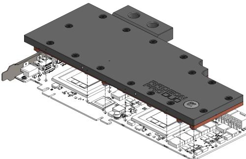
3. ATTACHING THE BLOCK TO THE GRAPHIC CARD. Use a Philips screwdriver screw with the enclosed 18 (eighteen) M2.5x4 AX1 screws. EKWB recommends users to start tightening the screws around the GPU core and continue outwards. <u>Always use</u> a plastic washer under each and every screw! If the washer is already present on the circuit board (usually around the four GPU core screw holes) there is no need for additional washer.
