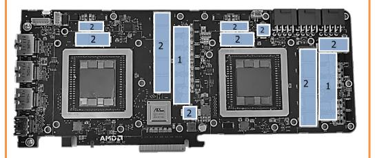
2. PLACING BLOCK TO GRAPHIC CARD. Carefully position the water block with preinstalled 2.5mm standoffs on to the graphics card. During this process please make sure you align mounting holes on PCB with holes on the water block. Also pay attention not to use too much force by pressing block down to PCB. Chip dies are prone to cracking.
