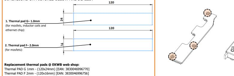
Place the M2,5 self-adhesive PVC washers under marked standoffs on monoblock and heatsink!
