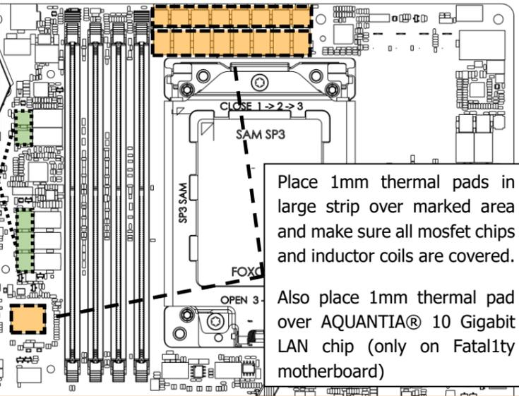
Place 1mm thermal pads in large strip over marked area and make sure all mosfet chips and inductor coils are covered.
