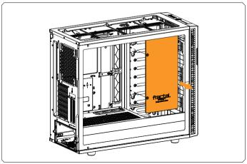
You can also remove the drive cover in order to secure the distribution plate with additional mounting screws if required.
